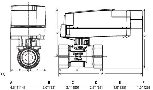
Modulating, Electrical fail-safe, 24 V
